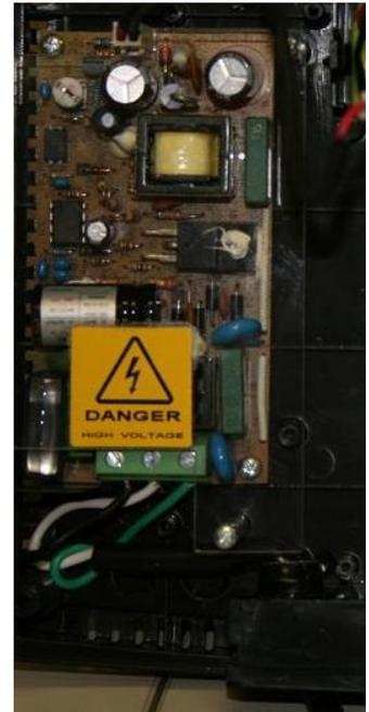
8. Remove the power cable by loosening the 3 screws for the black, white and green wires and pulling them from the connectors. Remove the power cable from the unit.
