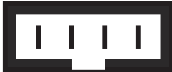
Figure 4-3: J4 - RS-232 Jack Pinout
